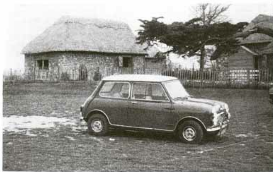
at the Roman Villa site at Bignor, near Goodwood, Sussex. The light alloy Gran Turismo wheels increase the track as well as reduce the unsprung weight. Dunlop SP41 tyres provided 60 per cent. extra mileage
