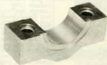
Steel centre main bearing cap, partly finished
