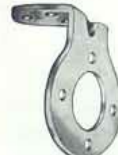
1634 Diameter of plate 3 1/2" Diameter of centre hole 1 1/2" Pitch circle diameter 2 1/2" Base length 2 1/2" (For use with lamps 1594, 1595, 1626 and 1627).
