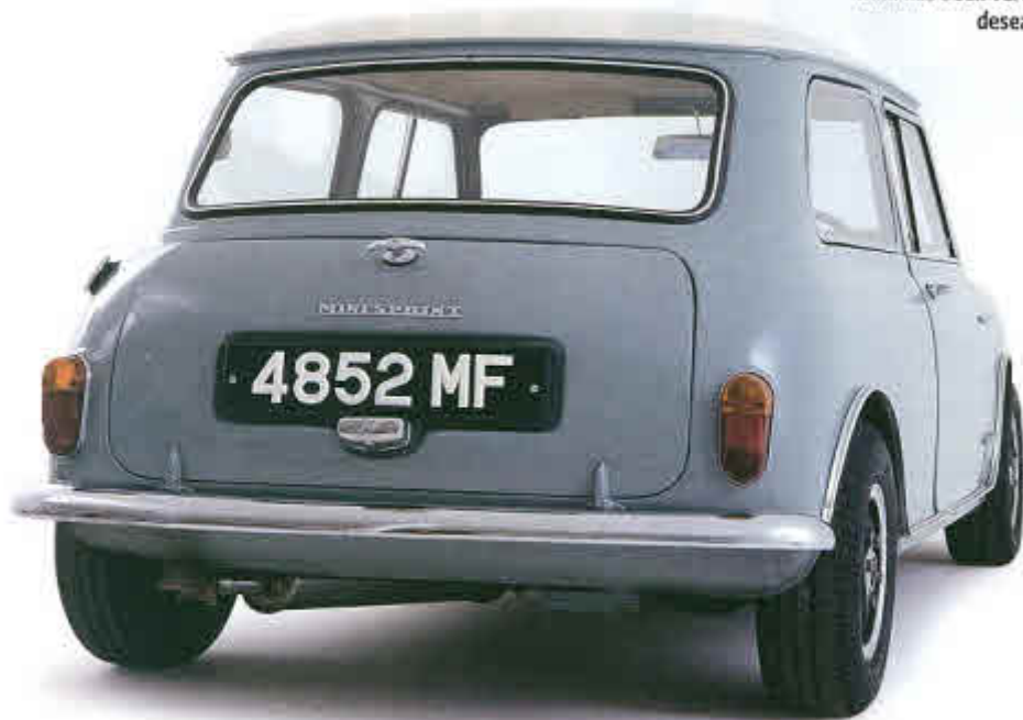
Along with the chop, the Mini has been vertically deseamed.
