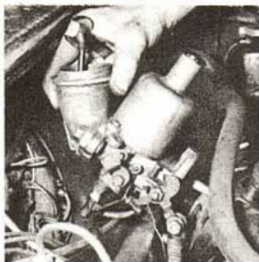
First remove the air cleaner prior to detaching all carb controls. Unbolt the SU from the inlet manifold studs and remove unit from engine
