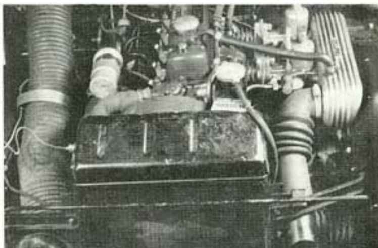
ENGINE CONVERSION SHOWING COLD AIR BOX
