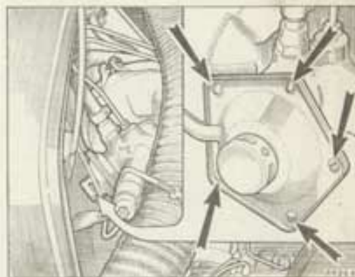
Indicating the retaining screws for the air valve cover and location of the servo
